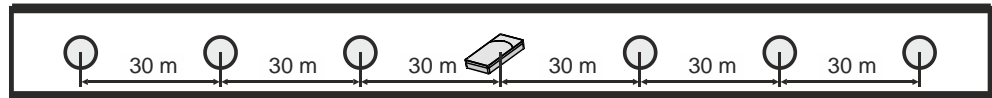
Figure 3: Radio gateways and radio devices in a multi-story building without intermediate walls
